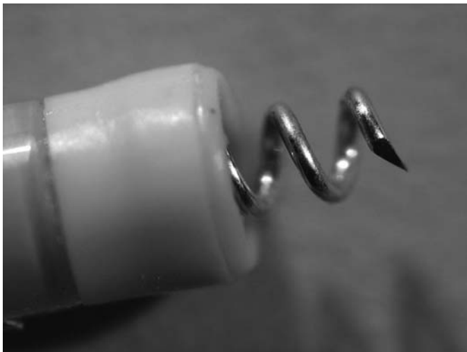
FIG. 1—Screw-in tip of Guidant atrial pacemaker lead \times 25 .
